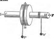
these pivots which rest in fixed sockets. A cord coiled round the wheel has one end fastened to the wheel, and at the other end the power (P) is applied. Another cord coiled round the axle in the opposite direction has one end fastened to the axle, and the other attached to the weight (W).
